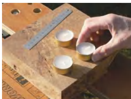
▲ Pic.2 ...then position several tea-lights on the hardwood block to give some idea of spacing. This is important if you want to end up with a regular geometric pattern!
